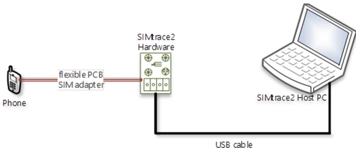
Figure 6 below shows a physical setup for the SIMtrace device.
